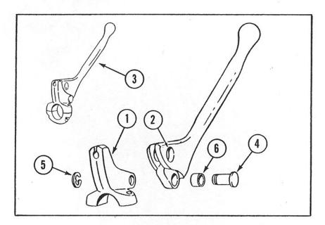
Above kits contain the latest bracket (Item 1) having a smaller 13/32 dia. hole as used with latest handlevers. A bushing (Item 6) is included, which fits into larger hole in your old lever (Item 2) to accommodate a smaller pivot pin (Item 4) and retaining ring (Item 5), also included in kits.
