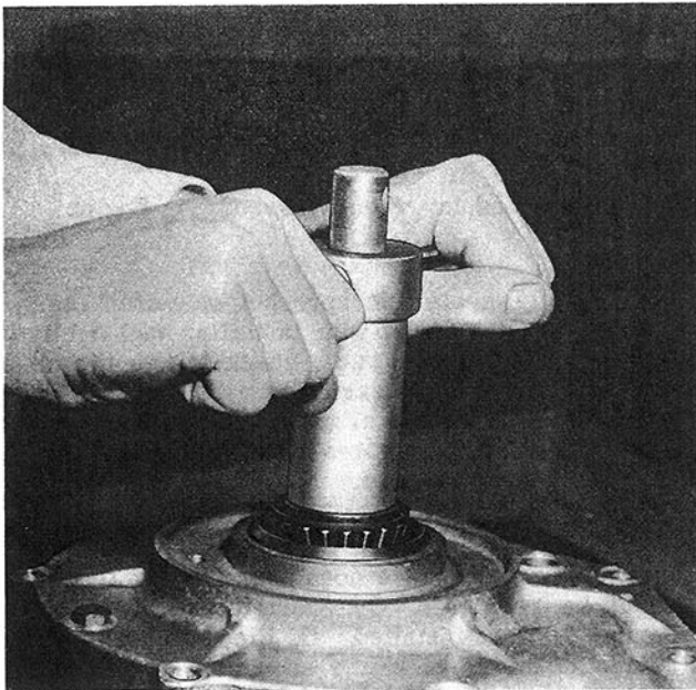
Figure 3. Assembling Flywheels into Sprocket Side Crankcase
