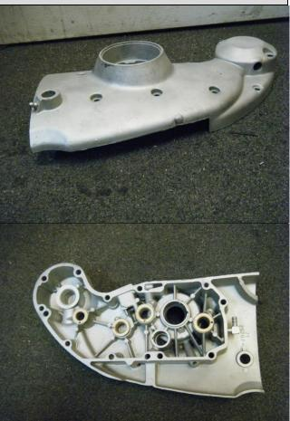
25201-71, XLH Models 1971-\* 25201-71, 71-\* XLH. First XLH with a horizontal "Circuit Breaker". Has notched out area for electric start.
